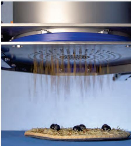
Our spice dispenser is an essential unit for a pizza production line. Extremely simple to use and wash, it enables you to measure out dried spices (oregano, basil, paprika, etc.) onto pizza bases. The dosing is very precise and homogeneous.
