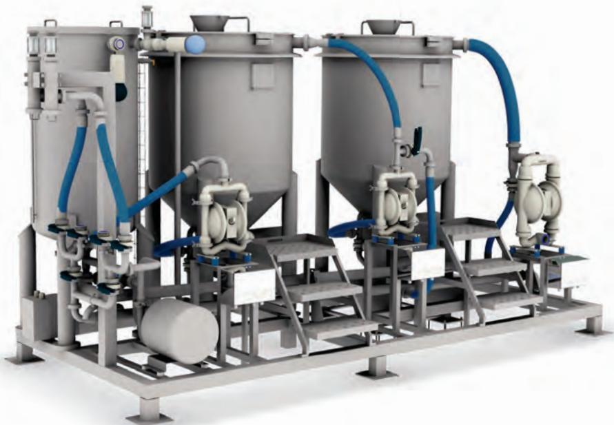
Our mixing and preparation unit for tomato sauce is designed for mixing tomato paste with fluids (water, oil, etc.) and spices.
