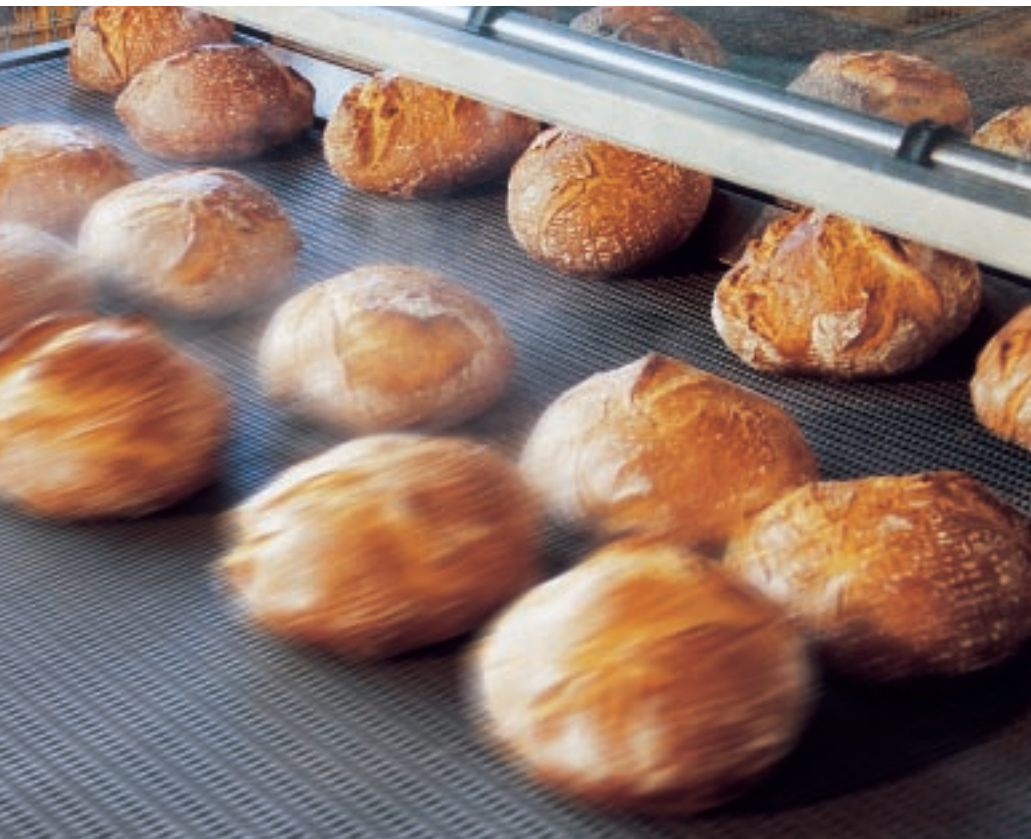
Spraying the baked products with a standard spraying device or pneumatic water atomizer
