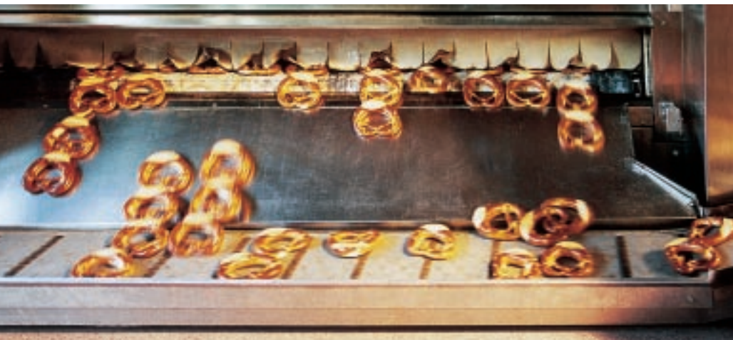
Baking oven outlet with chute and cross conveyor belt
