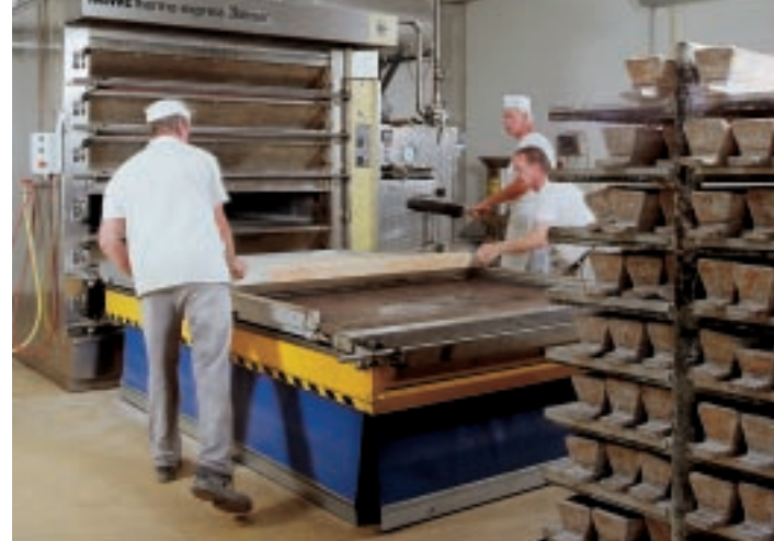
Patented pull-out trolley with variable working height for good ergonomics at all times
